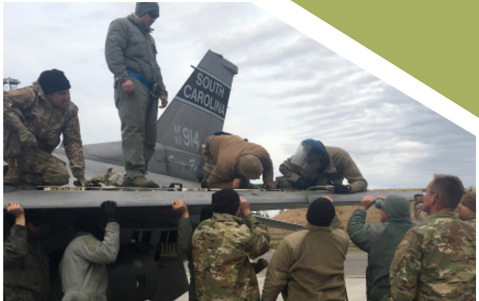
U.S. Air Force F-16 aircraft maintainers, assigned to the South Carolina Air National Guard's 169th Fighter Wing, remove the right wing leading edge flap after the discovery of a damaged actuator on one of their F-16 Fighting Falcons during Arctic Challenge Exercise 2019 at Kallax Air Base, Sweden, May 23, 2019. (U.S. Air National Guard photo by Lt. Col. Brian Doyle)
